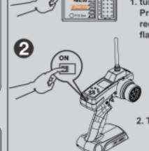
turn on the receiver power. Press the SW switch. The receiver's LED should start flashing.
